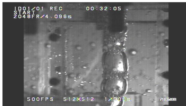
Figure 3: Zoomed-in view of the separation action in the DYNASWIRL® phase separator during the low-g period of a parabolic aircraft flight. The horizontal scale of the field of view corresponds to approximately 10 cm.
